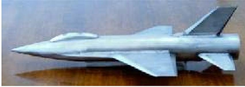
Figure 1- The Standard Dynamic Model (SDM)
