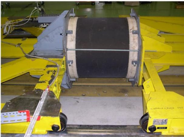
Fig. 3. Shell on the experimental equipment before the dynamic buckling test.
