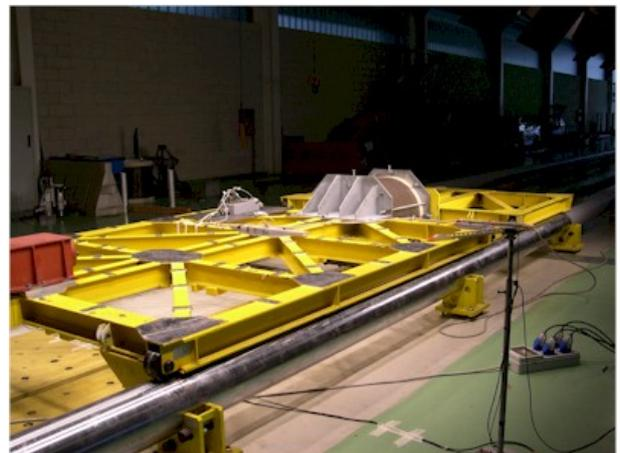
Fig. 7. Configuration of the crash equipment prepared for the dynamic buckling test.
