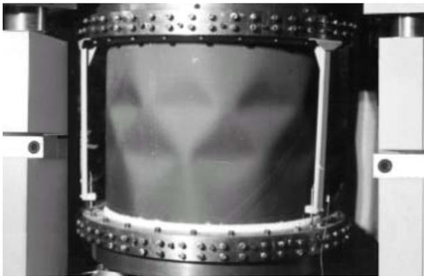
Fig. 2. Post-buckling mode of the axial compression static test.
