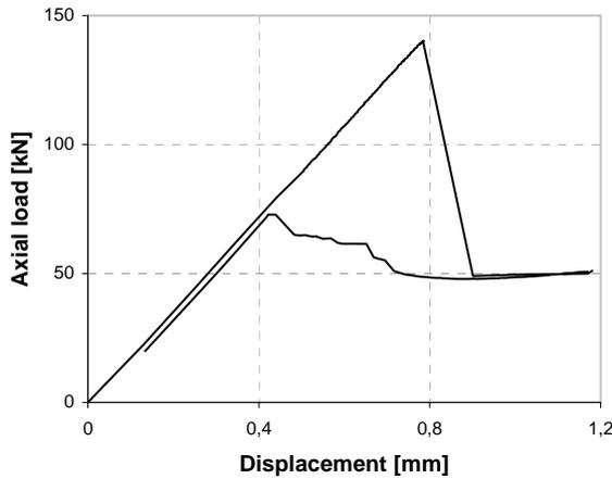
Fig. 1. Static test: diagram of axial load versus displacement.
