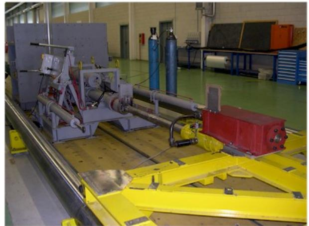
Fig. 6. Pre-calibrated hydro-pneumatic brake.
