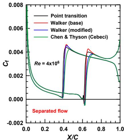
Fig. 7. Evolution of the skin friction coefficient using transitional flow models for  $Re = 4 \times 10^6$ .
