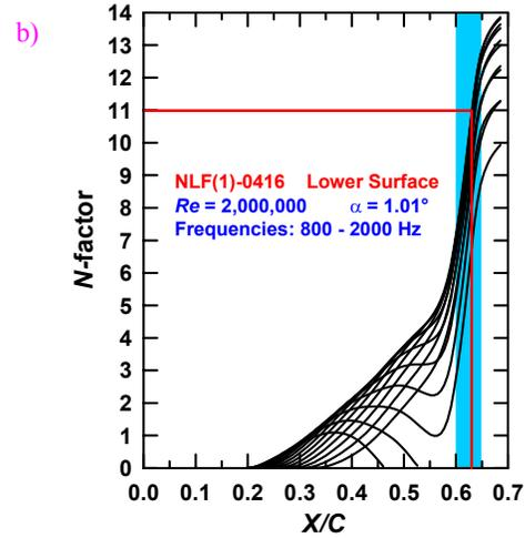
Fig. 3. Predicted transition locations using point transition for  $Re = 2 \times 10^6$ :
