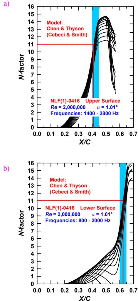
Fig. 6. Predicted transition locations using Cebeci and Smith version of Chen and Thyson transitional model for  $Re = 2 \times 10^6$ :
