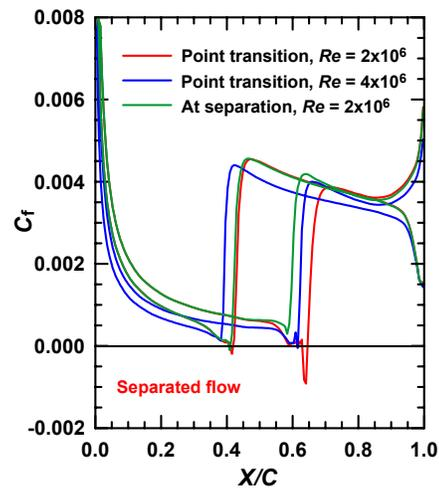
Fig. 4. Evolution of the skin friction coefficient using point transition.
