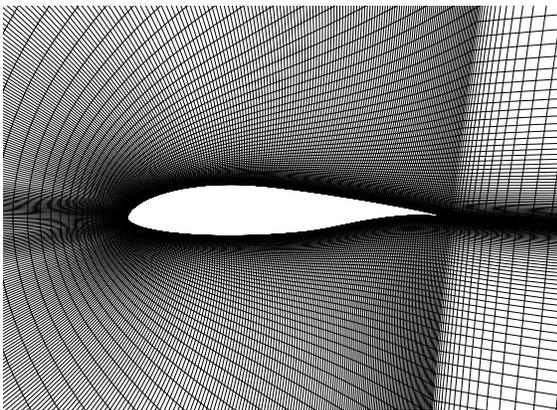
Fig. 1. Airfoil geometry and numerical mesh.
