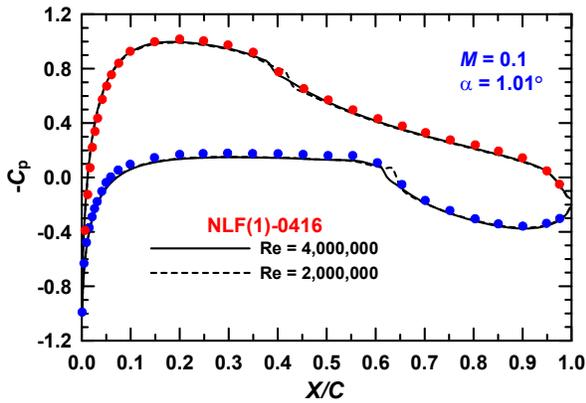
Fig. 2. Numerical predictions of the pressure distribution using point transition (symbols denote experiments).
