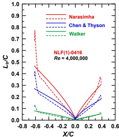
Fig. 5. *A priori* evaluation of the transition length generated by the various models at  $Re = 4 \times 10^6$ .
