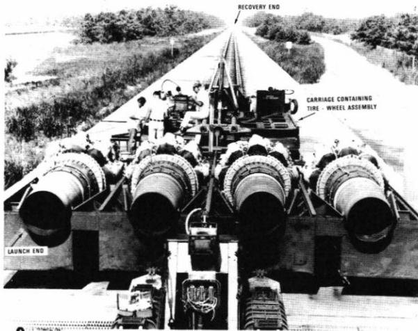
FIGURE 1. JET-POWERED VEHICLE AND ASSOCIATED SYSTEM
