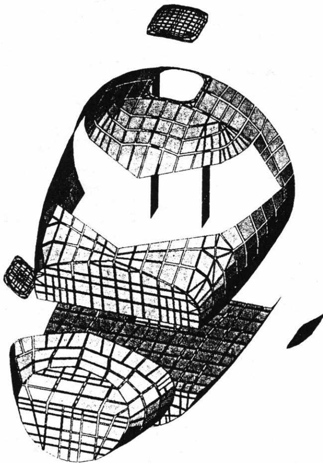
Fig 8 FE-model of SF-340 cockpit part of fuselage. Reproduced in grey-scale.
