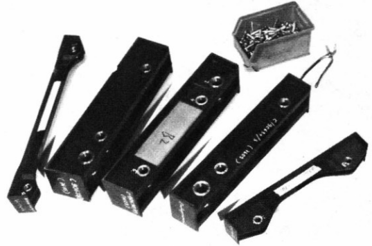
Fig.8 CFRP rudder support fittings
