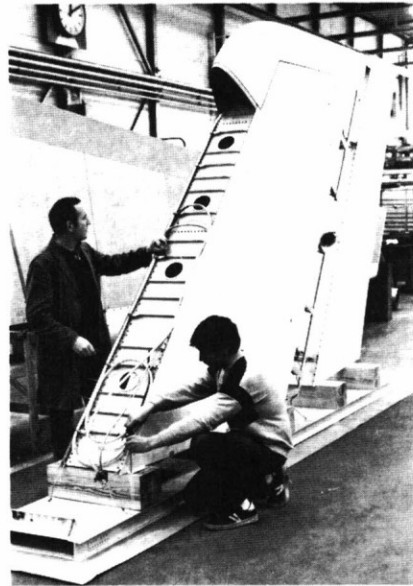
Fig.22 Lightning strike test specimen
