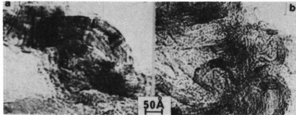
Fig. 11 – Lattice-fringe images of transverse sections of Celion GY 70 : a) area near fibre surface ; b) area near the core.
