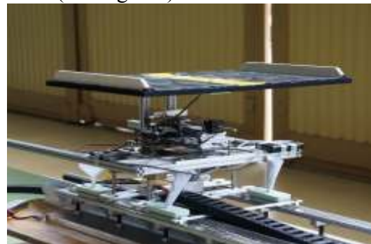
Fig. 11. Maglev track with sledge and landing platform
