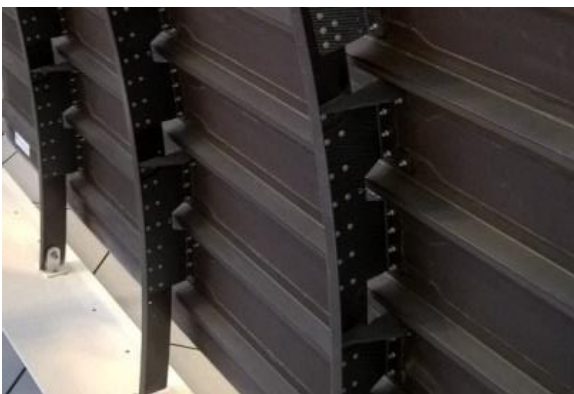
Fig. 3. Airbus A350 stringer fuselage structure [11]
