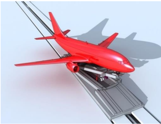
Fig. 2: Gear-less aircraft on acceleration/deceleration vehicle [8]
