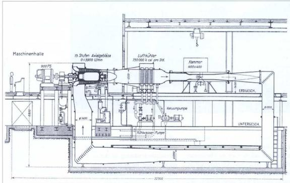
Fig. 8: The first closed-cycle supersonic wind tunnel at the ETH in Zurich, 1934.
