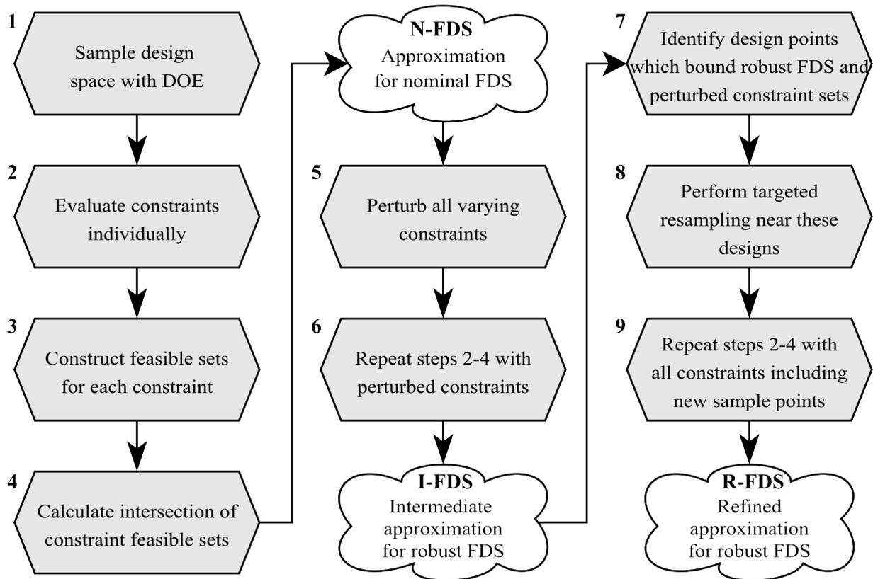
**Fig. 2** Dynamically Constrained Set-Based Design Methodology Flowchart
