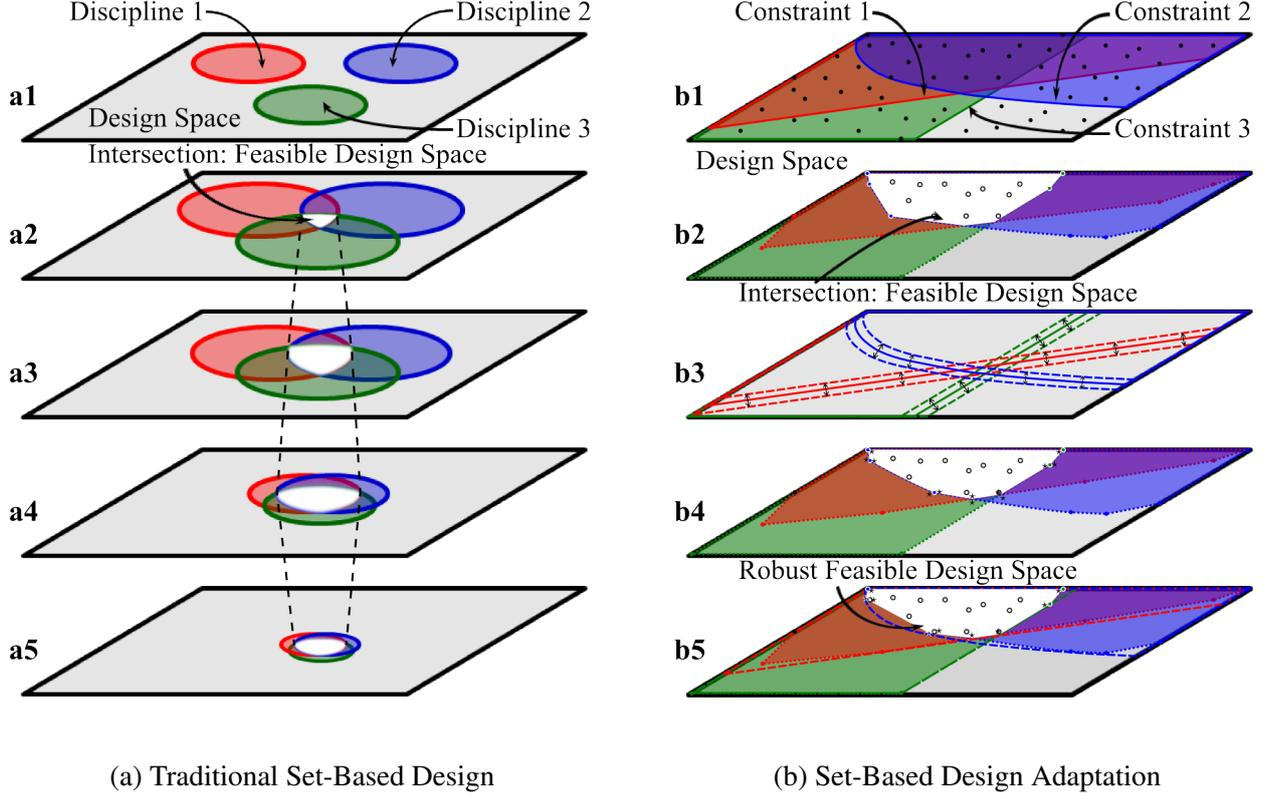
**Fig. 1** Set-Based Design: Traditional Process vs. Dynamically Constrained Set-Based Design
