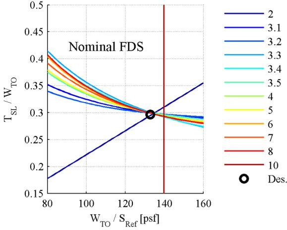
**Fig. 3** LTA design space visualization through energy-based constraint analysis
