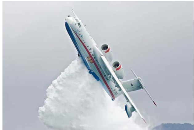
Fig. 4. Wildfire Water Drop Performed By The Be-200ES Firefighting Aircraft At Maneuvering In Mountainous Area
