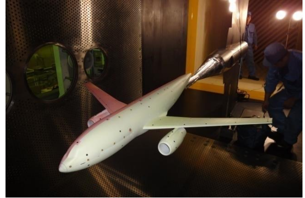
Fig. 12 DLR-F6 model mounted in the test section of JAXA TWT1.
