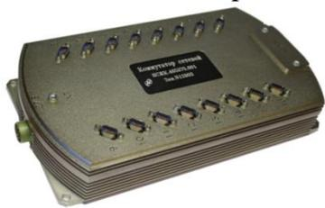
Fig. 6. 16-port SpaceWire routing switch for airborne networks
