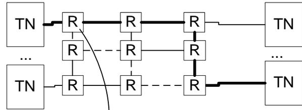
**Fig.3 Adaptive routing by routing table**
