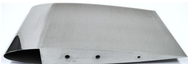
**Figure 5. NACA 0012 airfoil with the ultrasmooth nanostructured hydrophobic surface in the leading edge area.**
