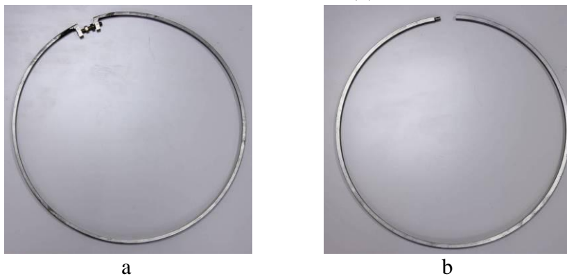
Figure 4 – Ring dampers No. 1 – (a) and No. 2 – (b) for blisk and its expanding devices
