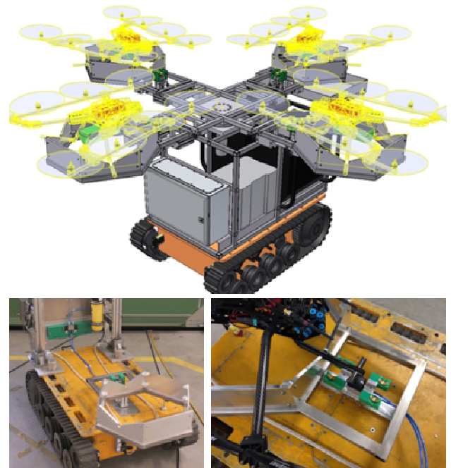
Fig. 1: Mobile transport system with landing platform and recharging contacts 2
