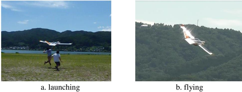
Fig. 14 Flight test of the solar plane
