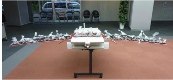
Fig. 4 Static load test for structure
