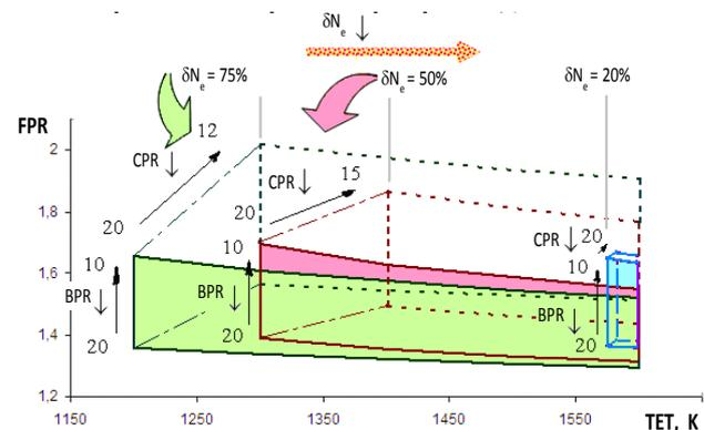
Fig. 4. Cruise design parameter ranges of HGTE-1 for kerosene ( $R=1200$  kgf,  $H=11$  km,  $M=0,78$ )
