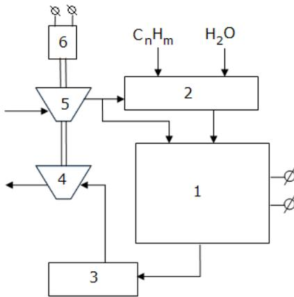
Fig. 3. The scheme of the PU based on SOFC and kerosene autothermal reforming
