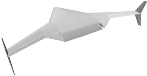
Fig. 12 Model No 8 with deflected inner flap
