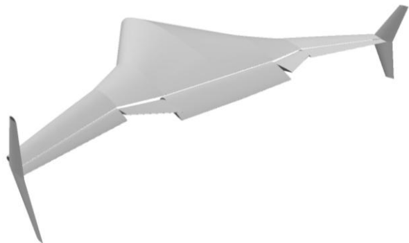
Fig. 13 Model No 8 with deflected middle flap
