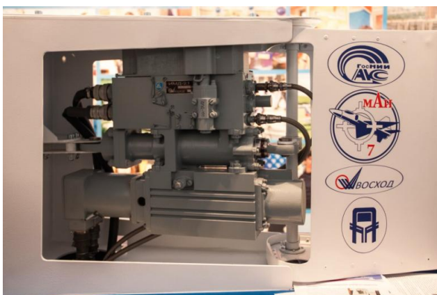
Fig. 4 Demonstrator of a hybrid electrohydraulic actuator with combined regulation of output speed
