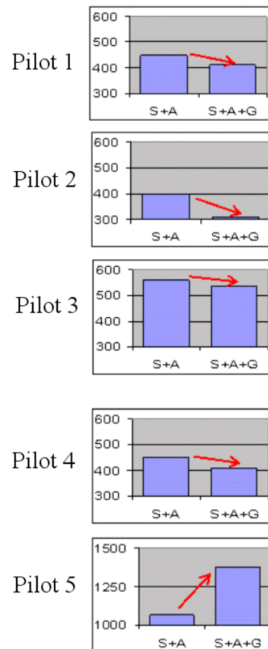
Fig. 13. Effect of G-load indication on the altitude loss while aircraft upset recovering.
