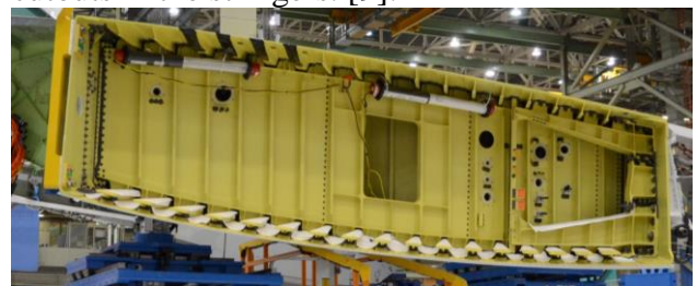
Fig.2. Wingbox root section of Boeing 787 Dreamliner [11]
