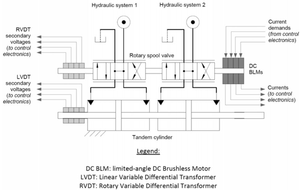
Fig. 1. Fault-tolerant actuator for fly-by-wire helicopter.
