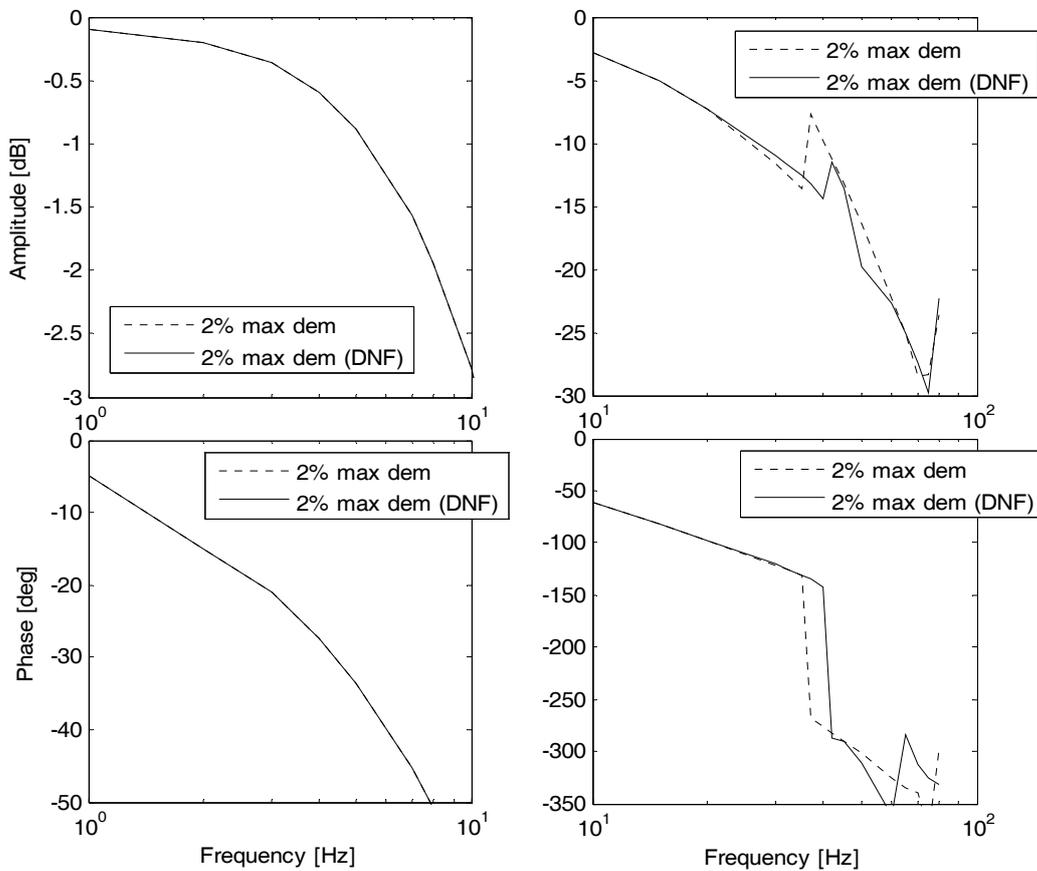
Fig. 8. Effects of the DNF on the actuator closed-loop dynamics (1 active coil).
