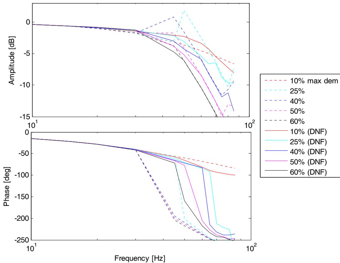
Fig. 6. Effects of the DNF on the servovalve closed-loop dynamics (1 active coil).
