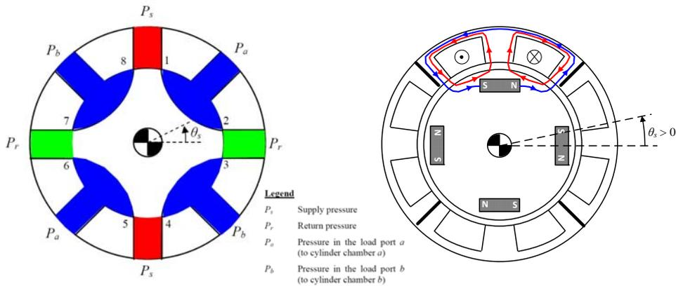
Fig. 2. Actuator servovalve: (a) single unit of the rotary valve; (b) limited-angle brushless motor.
