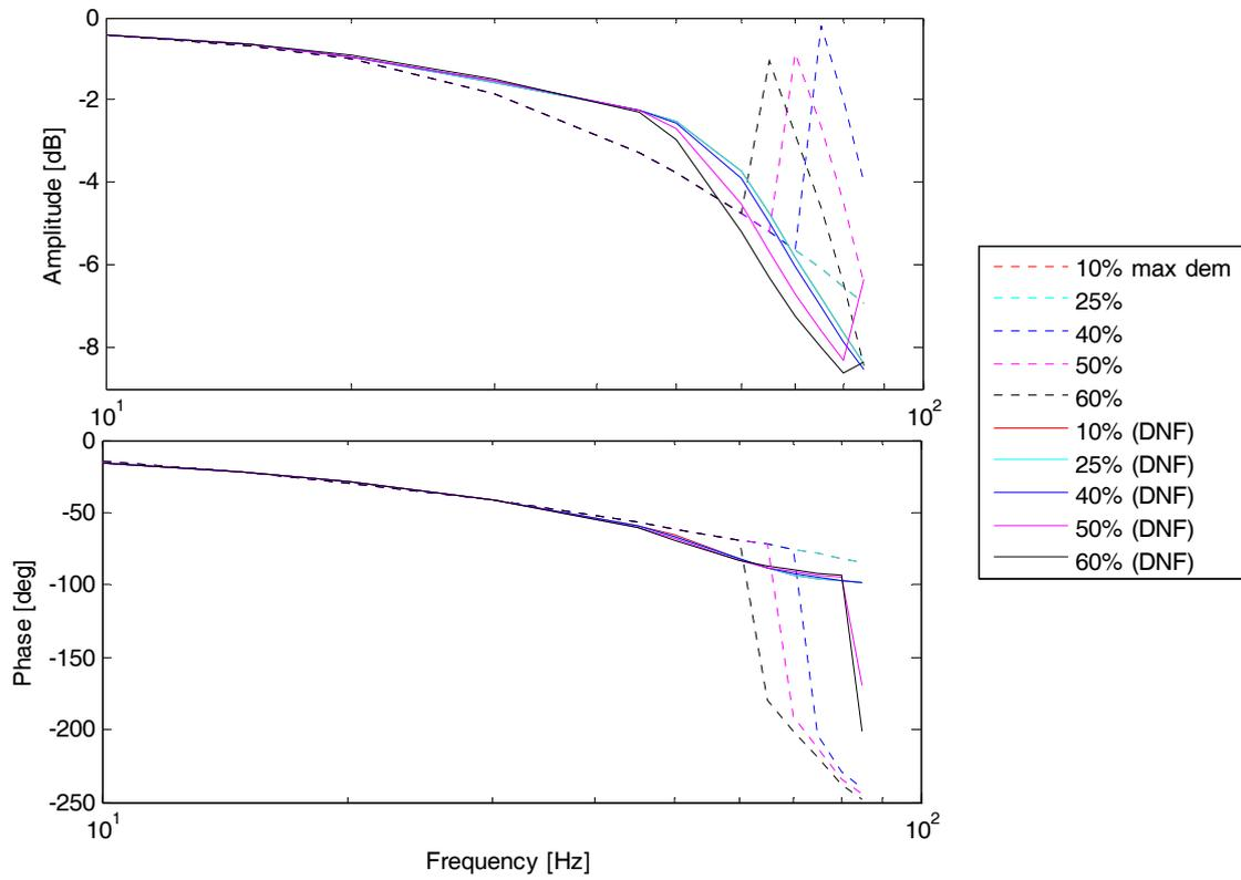
Fig. 5. Effects of the DNF on the servovalve closed-loop dynamics (3 active coils).
