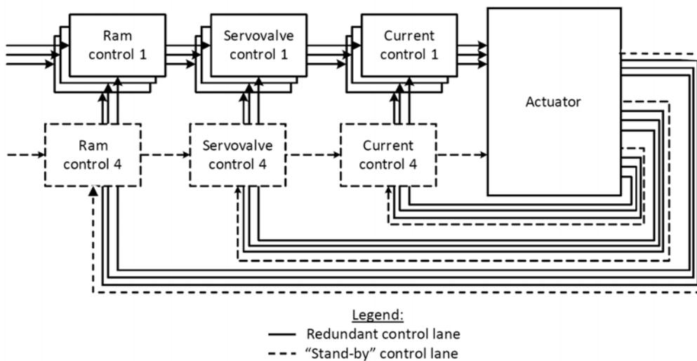
Fig. 3. Actuator closed-loop control scheme.
