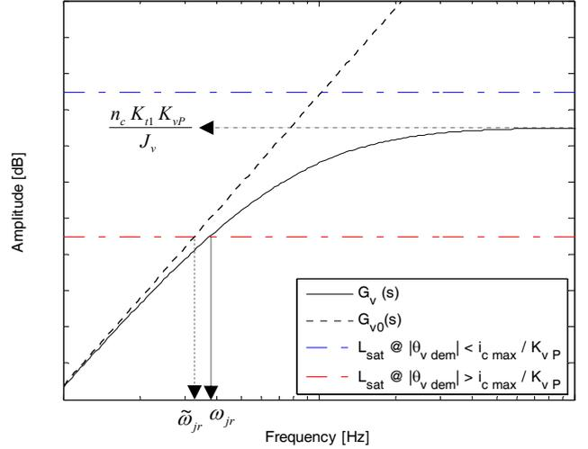
Fig. 4. Jump resonance frequency estimation.
