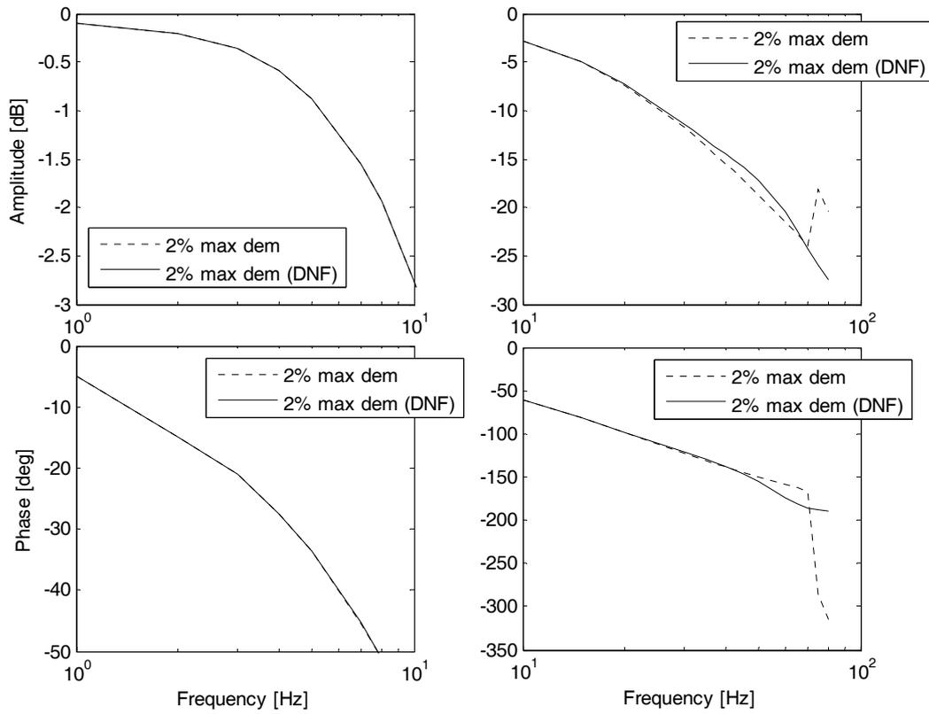
Fig. 7. Effects of the DNF on the actuator closed-loop dynamics (3 active coils).
