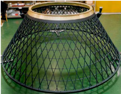
Fig.2 – Lattice composite structure of a rocket adapter
