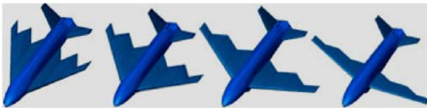
Figure 2. Biologically inspired morphing aircraft: sliding skin (Raytheon, sweep angle changes) [3].
