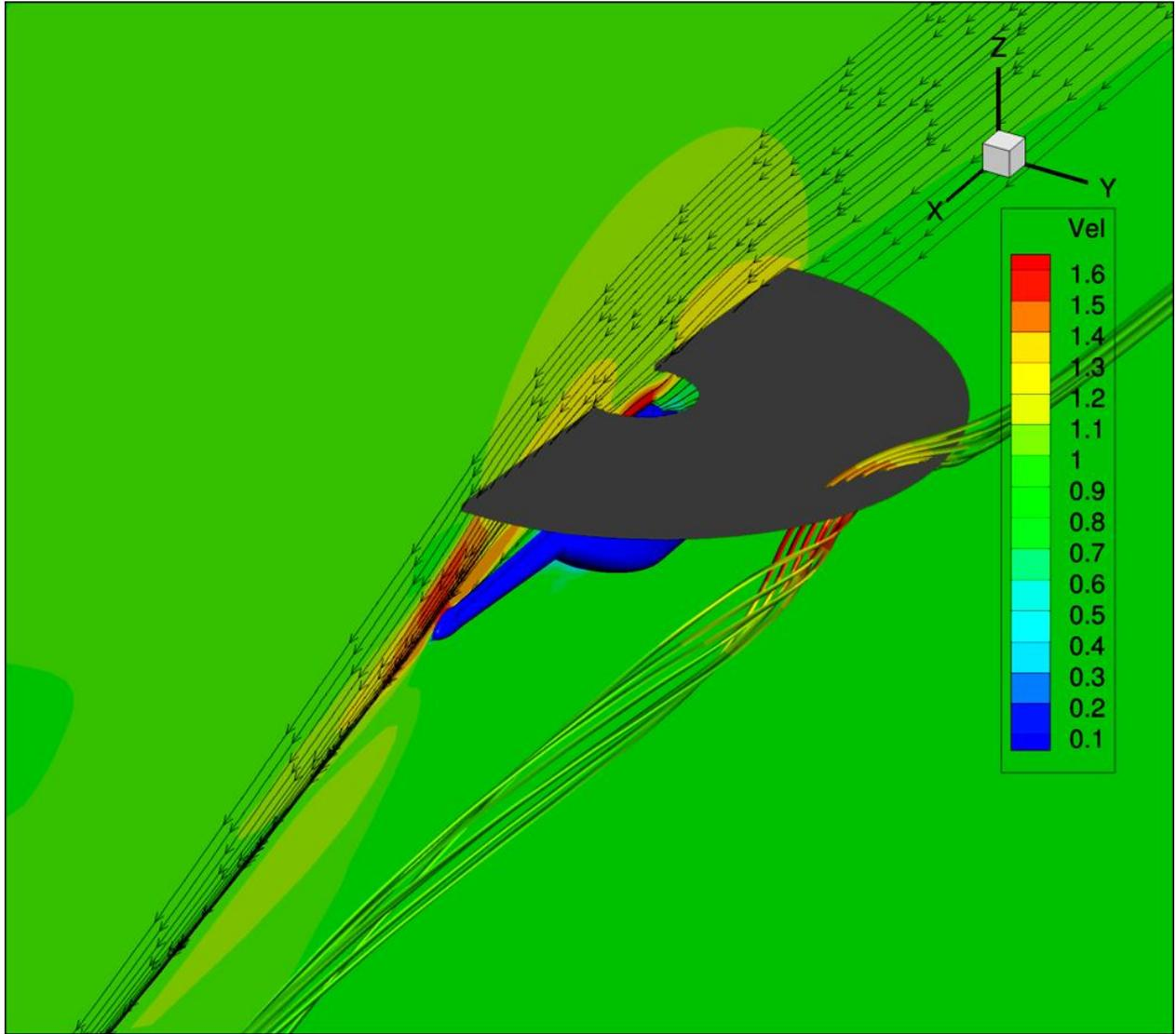
Fig. 1. Reproducible phenomenon: downwash and tip vortices
