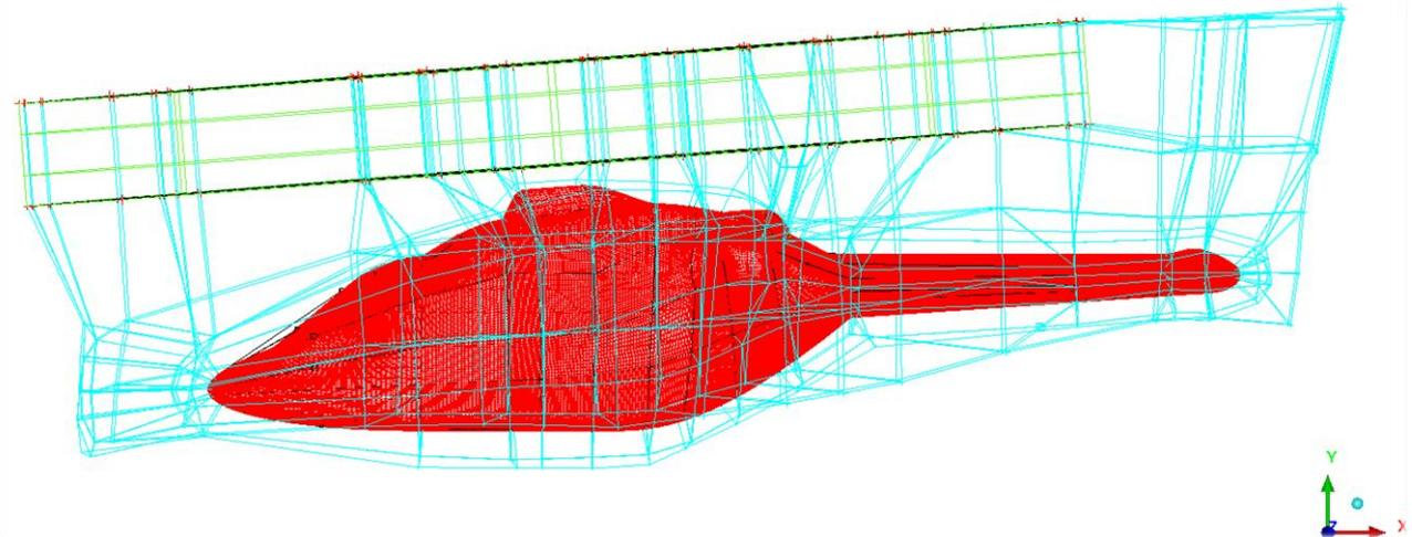
Fig.4. Blocking near the fuselage
