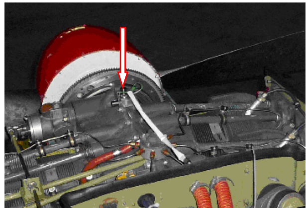
Fig. 2. Installation position for accelerometers on the engine
