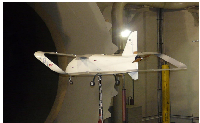
Fig.1 Joined wing demonstrator investigated in this project, in the wind tunnel.
