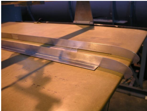
Fig. 16. Boundary layer fence installation on flat plate
