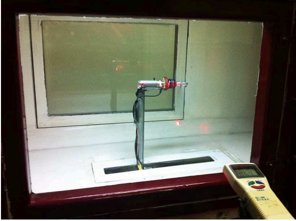
Fig. 4 Propeller Wind-Tunnel Experiment
