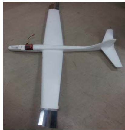
Fig. 24 Glider with primary feather wings
