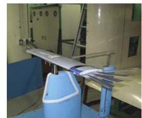
Fig. 4 Model with primary feather wings
