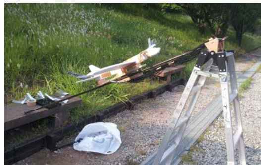
Fig. 26 Catapult launch system
