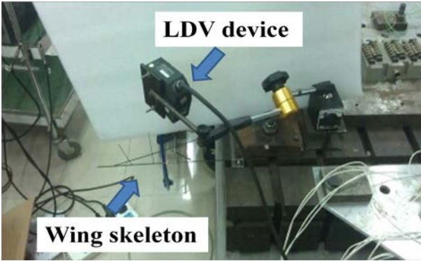
Fig. 6. Experimental Setup of LDV Device
