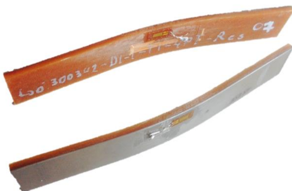
Fig. 14. Specimen, four point bending tests with GFRP 2.0mm basis laminate and 0.4mm titanium erosion shield after static test.
