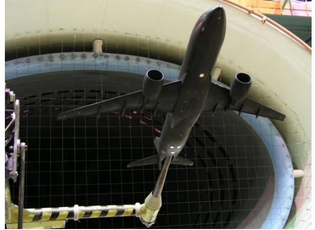
Fig.1. Wind tunnel dynamic tests of passenger aircraft.
