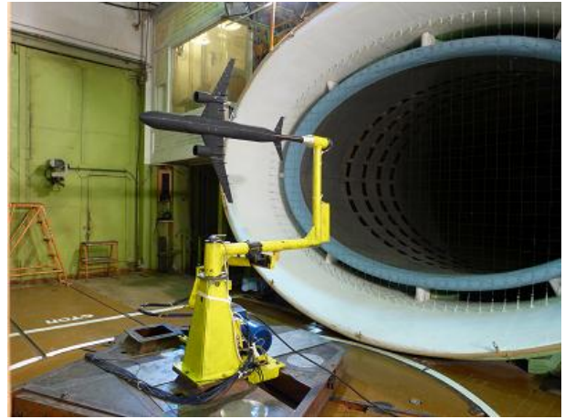
Fig. 6. The OVP-102B test rig in the working section of T-103
