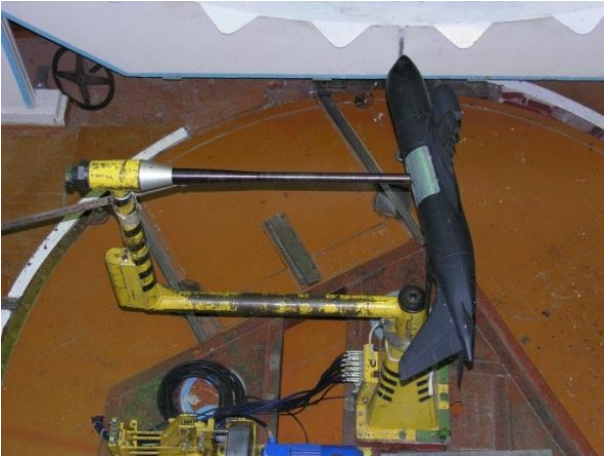
Fig. 9. The aircraft model on free oscillations test rig in the working section of T-103
