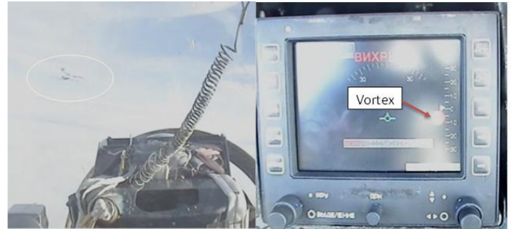
Fig. 2. View of wake-generator Tu-154M (left) via canopy of L-39. L-39 onboard LCD (right). H = 3170 m, Vias = 380 km/h, neutral atmosphere.
