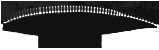
Fig. 7. Photograph of divided light bunch at upper surface of a model with flow.
