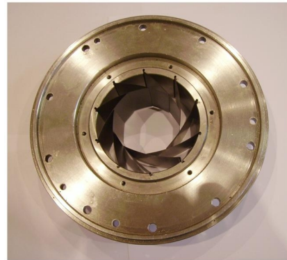
Fig. 3. Experimental foil bearing Ø90 mm
