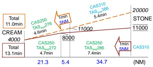
Fig. 9 Difference of flight time between CDO and STAR
