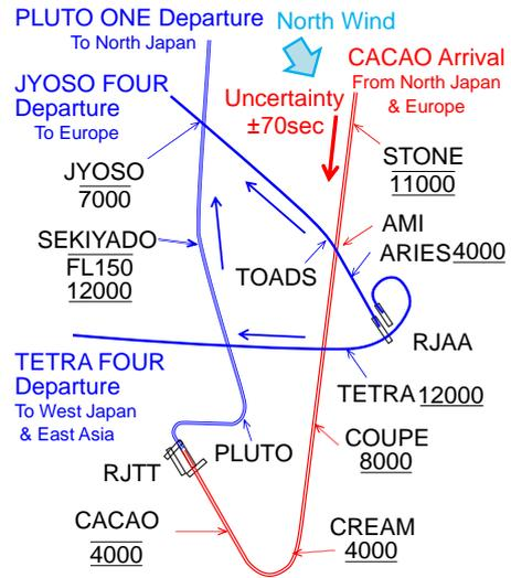
Fig. 7 Schematic of STAR and SID of RJTT and RJAA at north wind operation
