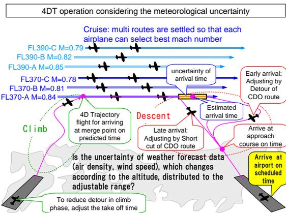
Fig 1. Concept of 4-Dimensional trajectory based operation considering the meteorological uncertainty
