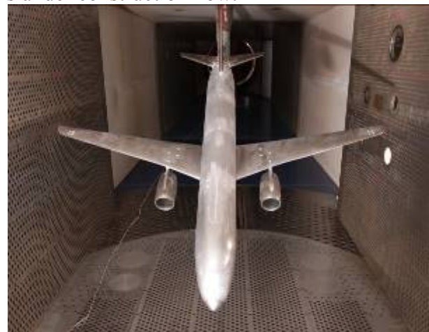
Fig. 12. Aerodynamic model of the regional jet with low-sweep wing in T-128 wind tunnel
