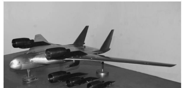
Fig. 6. TsAGI “flying wing” aerodynamic model with forward position of the upper nacelles
