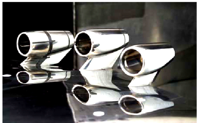
BWB model with pylon mounted nacelles.
