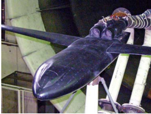
Fig. 8. Aerodynamic model of the regional aircraft with over-the-fuselage nacelles
