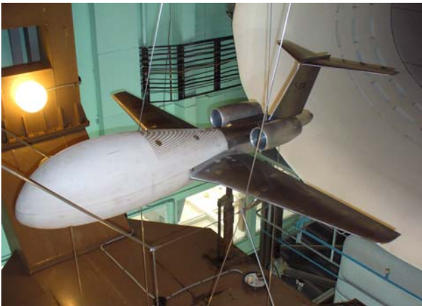
Fig. 2. The aerodynamic model in the low speed wind tunnel T-102
