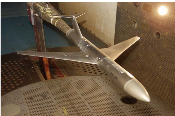
Fig. 8. Reference model in T-128 wind tunnel
