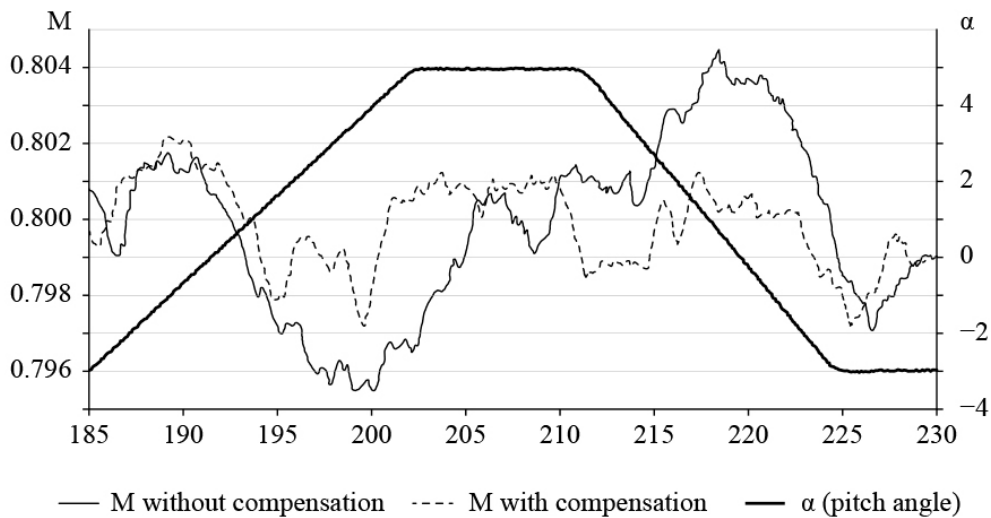
Fig. 5. M number stabilization in T-128 wind tunnel at the continuous variation of the aircraft model pitch angle with compensation and without compensation of the disturbing impact; \alpha – pitch angle
