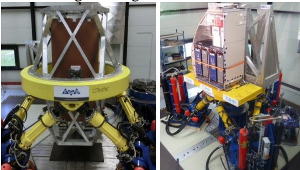
Fig. 2. Partition panel with literature pocket & magazine (left), fully loaded G2 galley (right) on 6dof shaker
