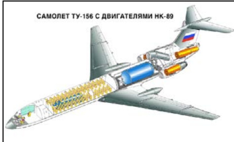
Fig. 3 Tupolev-156 airplane layout.
