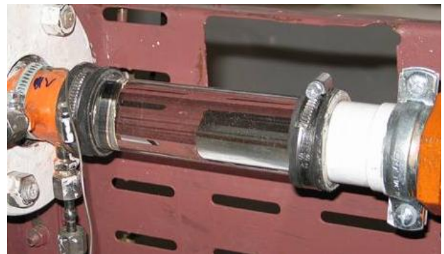
Fig.5 Fuel flow downstream of the diaphragm. P_0 = 60 kPa, T_0 = 293 K, U_0 = 0.65 m/s. Virtually no air released.
