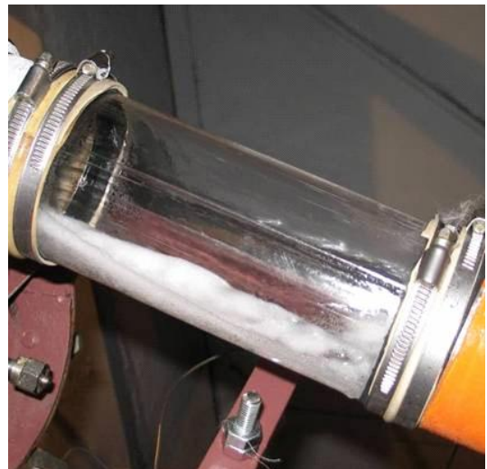
Fig.8. Two-phase flow in the tilted segment. P = 20 \text{ kPa} , T = 273 \text{ K} , U_0 = 0.71 \text{ m/s} , tilt angle 20 degrees.
