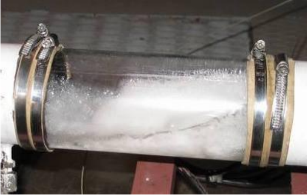
Fig.9 Two-phase flow after the tilted segment and the bend before the contraction. P = 20\text{kPa} , T = 273\text{ K} , U_0 = 0.64\text{ m/s} , tilt angle 20\text{ degrees} .
