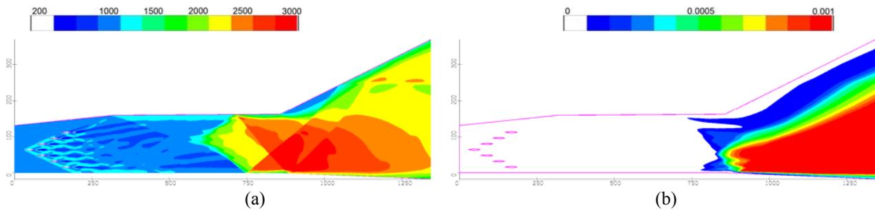
Fig. 1. Static temperature (a) and  $NO$  mass fraction (b) fields for model combustor in the case  $T_0=1100$  K
