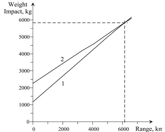
Fig 3 Weight load on the aircraft as a function of the flight range for conventional TFE (1) and hybrid TFE (2) based on SOFC battery with 2.5 kW/kg and  $\kappa_R = 2$ . Fuel is aviation kerosene.
