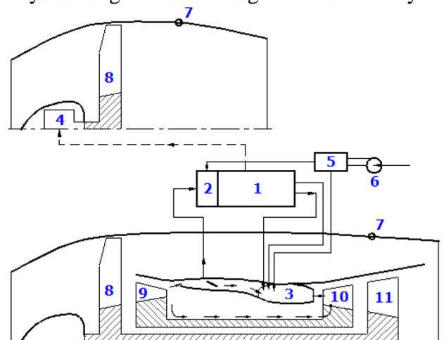
Fig. 1. The scheme of hybrid engine with the SOFC battery and the remote thrust fan. 1 - SOFC battery, 2 - Reformer, 3 - Burner, 4 - Electric motor, 5 - Fuel flow controller, 6 - Fuel pump, 7 - Nozzle of low-pressure contour, 8 - Remote thrust fan, 9 - High pressure compressor, 10 - High pressure turbine, 11 - Low pressure turbine.
